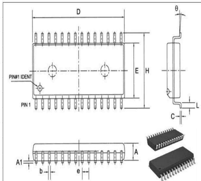
The diagram illustrates the physical dimensions of the SZY58F0 chip in a QSOP28 package. It includes a top view showing lead spacing (D), body width (E), body height (H), and a pin 1 identification mark (PIN#1 IDENT). A side view shows the thickness (θ), lead length (L), and lead pitch (C). Below the views are two photographs of the actual chip package.
