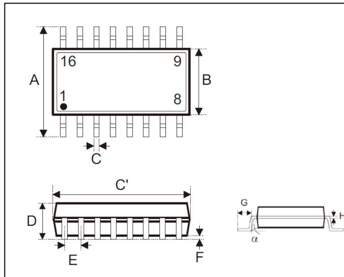
The diagram illustrates the physical dimensions of a 16-pin Plastic SOP package. The top view shows the package with pins numbered 1 through 16. Dimensions A and B represent the overall height and width respectively. The side view provides a detailed look at the lead profile, with dimensions C, C', D, E, F, G, and H defining various features like lead thickness and pitch. An angle symbol α indicates the lead angle.
